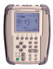
The IFR 6000 is a compact, lightweight and weatherproof unit designed for testing transponder modes A/C/S, 1090 MHz ADS-B and 978 MHz UAT, TCAS I and II, and DME. The IFR 6000 features an extremely easy to use interface where every parameter the user commonly needs to view is displayed on screen.
